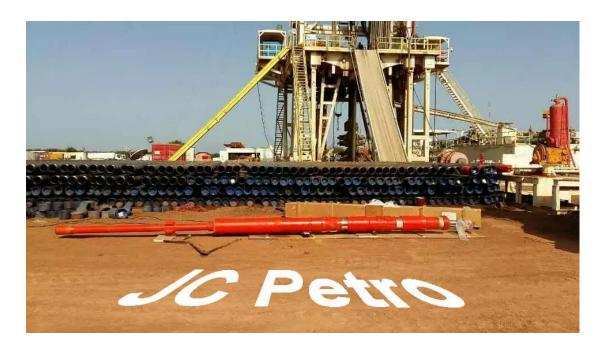
Casing cement head is widely used in the oilfield for cementing application, typically for pumping slurry and releasing plug. Our cement head includes single plug type, double plugs type, Multi-Plugs type, drill pipe type, etc. Our cement heads in various sizes and pressure ratings for superior performance in cementing operations.But today, we will introduce a high grade casing cement head ——-Top Drive Casing Rotating cement head.
